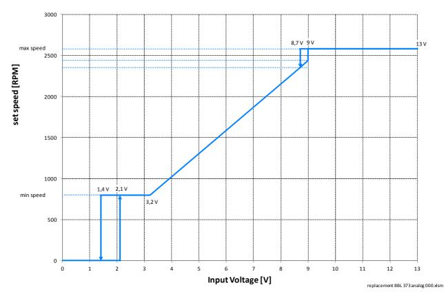
NOTE: tolerance on voltage threshold for minimum speed is 2.1 ±0.5 V
