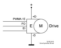
E stands for integrated electronics. M stands for motor. Drive stands for motor with axial integrated electronics.
