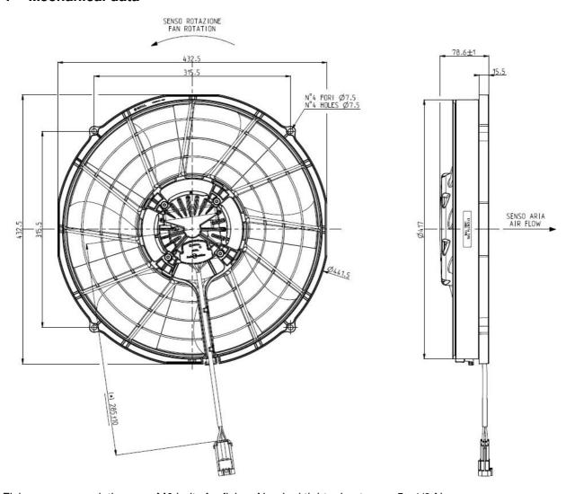
Fixing recommendation: use M6 bolts for fixing. Nominal tightening torque 5  $\pm$ 1/0 Nm Nominal torque defined for brand new, clean and lubricant-free bolts.
