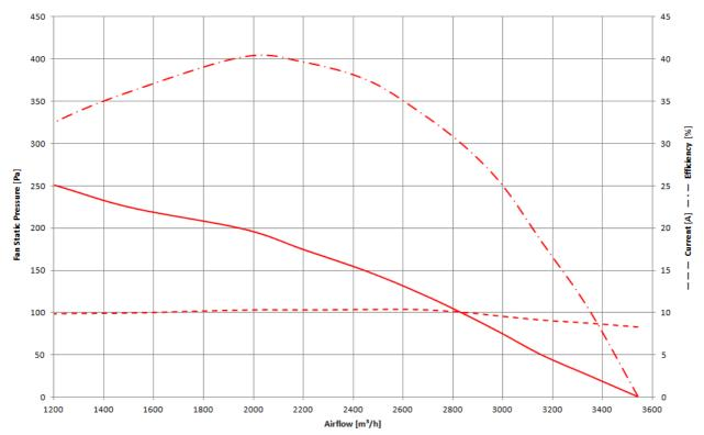
Air density 1.18 kg / m3 - Test number: #15009 - Test bench compliant to ANSI AMCA 210 TAMB = 20 °C ± 5 °C - UB = 26.0 V at the Drive connector
